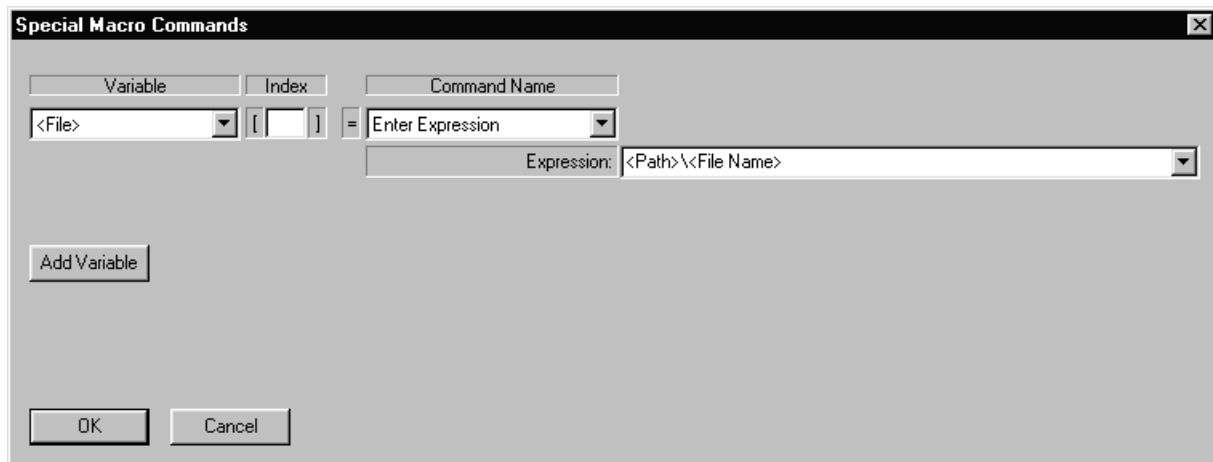
Figure 34: Assigning Variable Values Using Enter Expression
